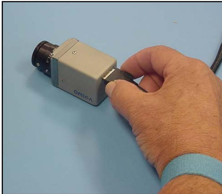
**Figure 4:** Connecting the Interface Cable to the Micron/A10
