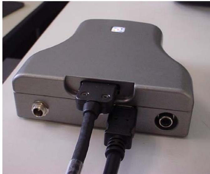
**Figure 16:** IEEE-1394 Cable connect to Firewire Module
